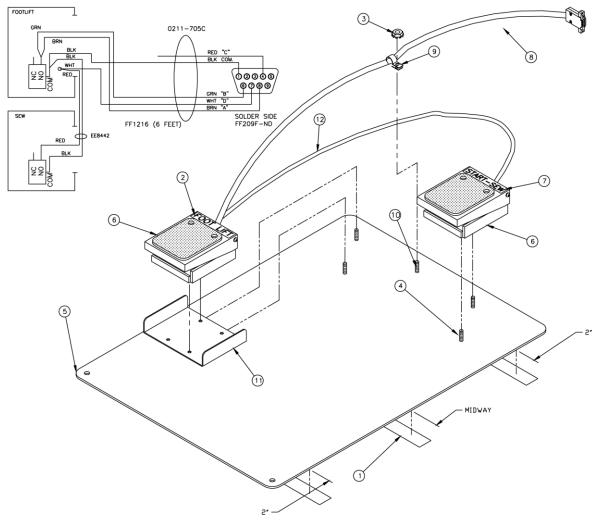
NOTE: THIS UNIT FOR USE WITH 1335MC TYPE UNITS ONLY. DO NOT PLUG DIRECTLY INTO EFKA CONTROL BOXES.
