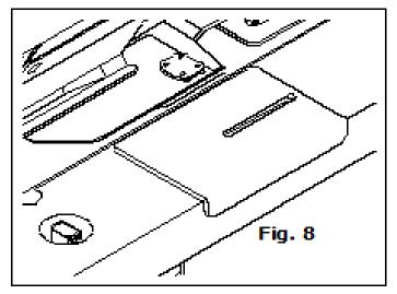
gusset through the folder, under the presser foot and under the puller. Load the panel under the gusset with the center of the short side even with the needle and the edge of the panel against the edge guide. Lower the presser foot. Be sure the Auto/ Manual switch is in its Auto position (up).
