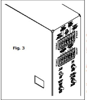
The Panels / Frames switch selects the operation mode. In the Panels mode the machine will detect the edges of a panel being sewn to the gusset and stop at each corner. In Frames mode no panel is used. The machine will sew for a specified preset distance, stop and make ruffles, and sew again until a four sided "frame" has been created.
